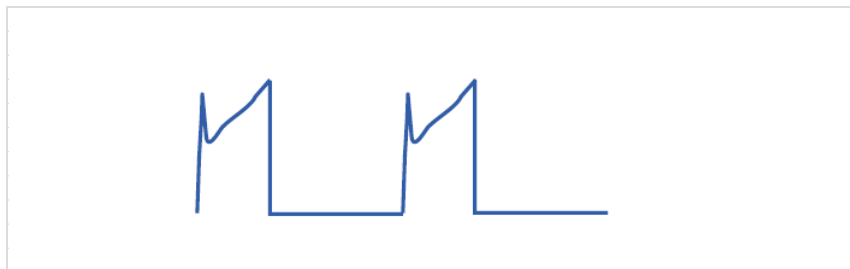
Figure 4.13 Practical circuit current-sensed waveforms [7]
